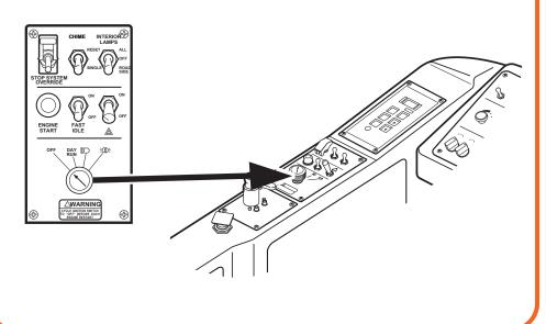
Turn off battery disconnect switch (Streetside, Front of Bus)
